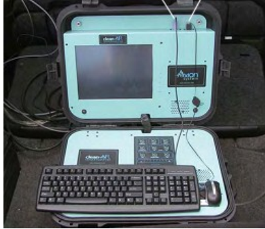
Figure 3.1 Axion Portable Emission Measurement System (PEMS)
